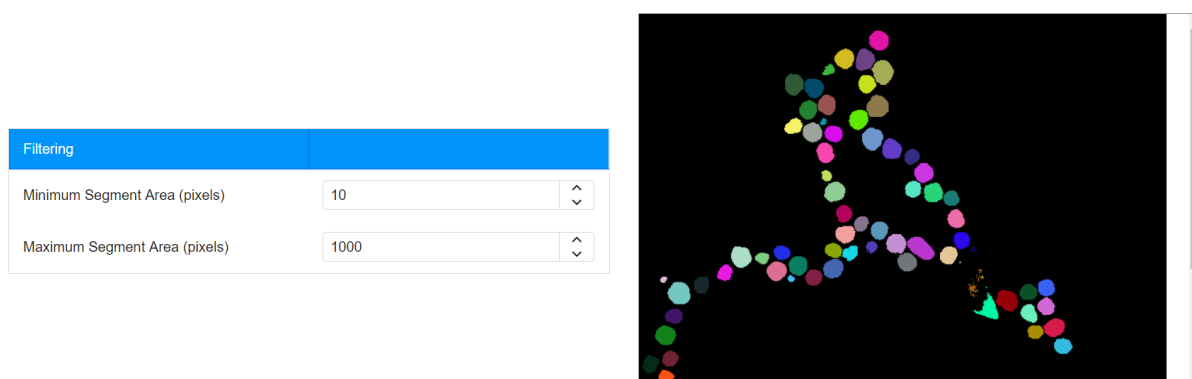
Figure 29: Filtering step. Removal of segments touching the border as well as removal of segments with less pixels than the minimum segment threshold and more pixels than the maximum segment area threshold.
